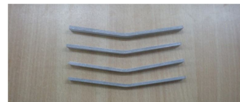
Figure. 7 specimen after Flexural testing
