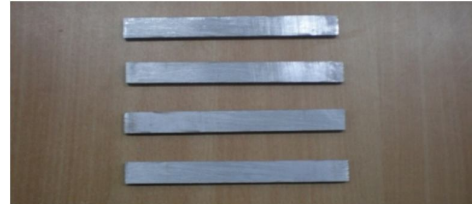
Figure. 6 specimen before Flexural testing
