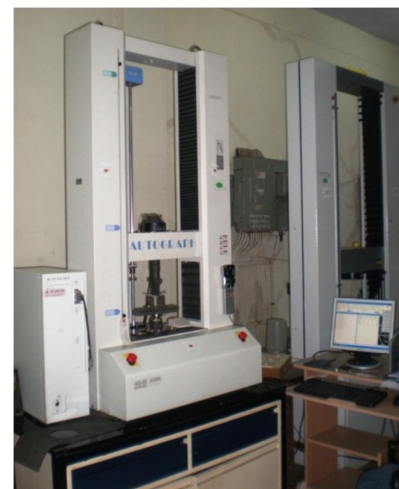
Figure. 9 Computer Controlled UTM Machine (SHIMADZU-50KN)
