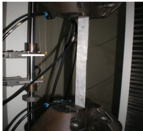
Figure. 5 specimen during tensile testing
